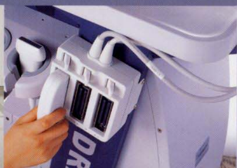
Cart supports three selectable transducers (Two active)
